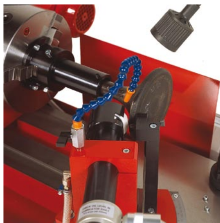
Water cooling system
